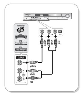
AV 3 IN selection will be automatically done. If the input is not selected automatically, use INPUT SEL. button to select proper input.
